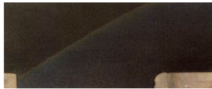
FIGURE 9. Flow visualization of the injectant using liquid-crystal thermochromic indicators.
